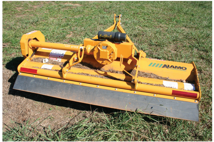
The flail mower finely chops and uniformly distributes plant residue on the soil surface.
