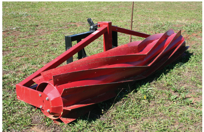
The roller crimper, with angle iron blades, crimps the stems and lays the intact plant uniformly on the ground.
